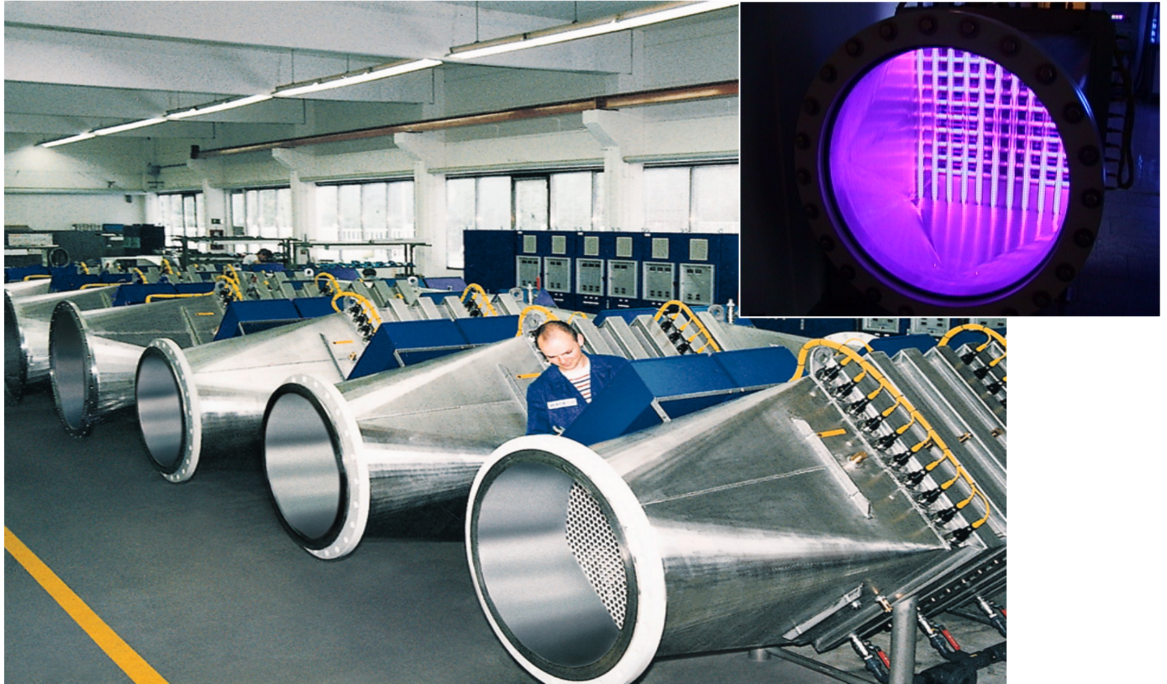
UV disinfection drinking water facility in Helsinki, Finland (Wedeco)
